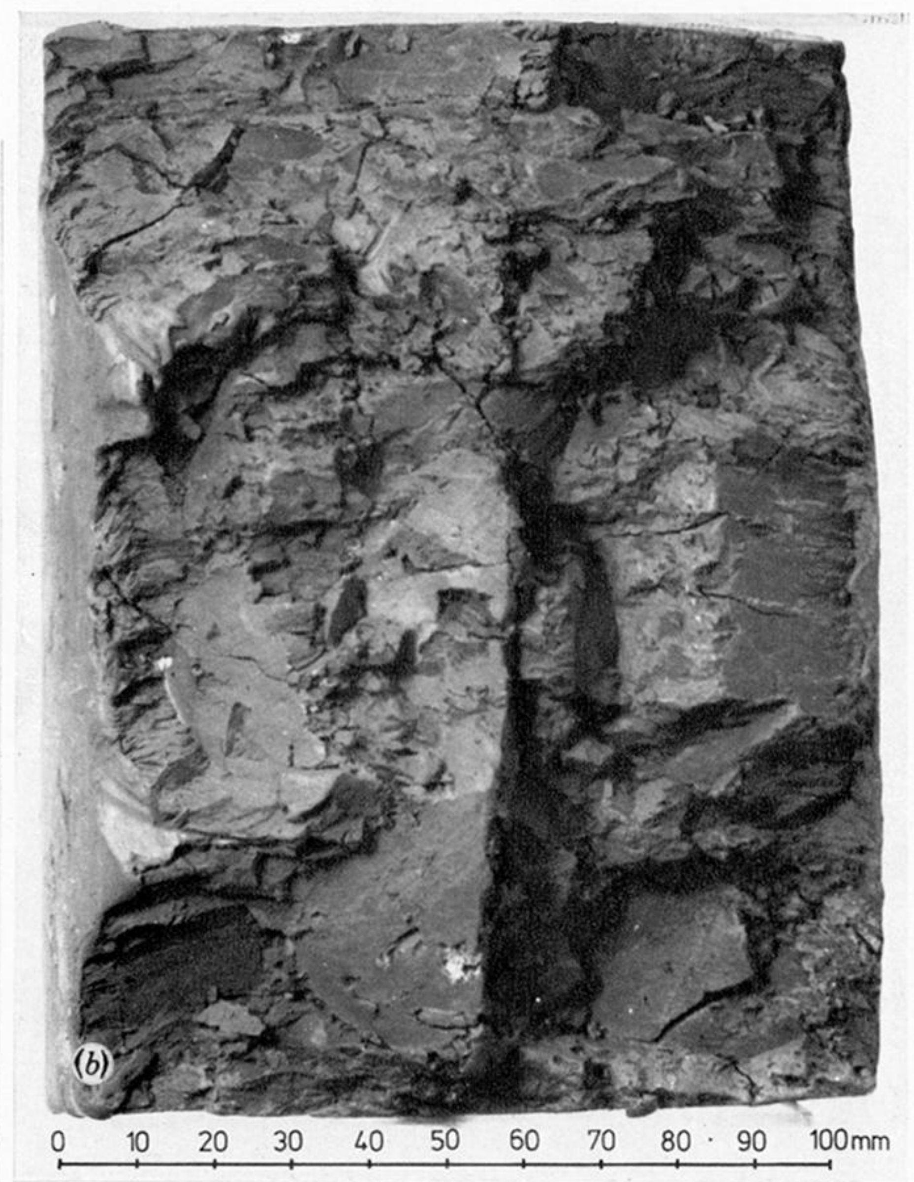
FIGURE 16. Photographs of hand specimens of different weathering zones of the London Clay. (a) Zone I (unweathered), (b) zone II and (c) zone IIIb.
